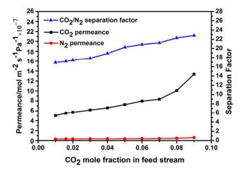
Fig. 3 Effect of the  $CO_2$  feed composition on the permeance and  $_5$  separation factor for  $CO_2/N_2$  binary mixture through the CAU-1 membrane at 298 K with a feed pressure of 0.1MPa.
