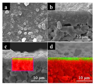
**Fig. 1** SEM image of the surface and cross-section of CAU-1 membrane (a, b) and EDS mapping of CAU-1 membrane: green C; red Al(c, d).
