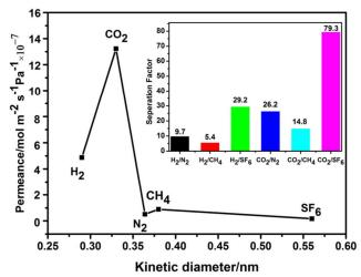
Fig. 2 Single gas permeances of  $H_2$ ,  $N_2$ ,  $CH_4$ ,  $CO_2$  and  $SF_6$  through the CAU-1 membrane and the ideal separation factors for the corresponding gas pairs
