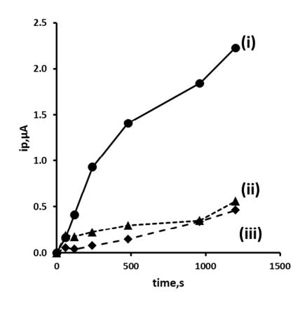
**Figure 5.** Effect of deposition time on the magnitude of stripping peak current for Pb. Deposition potential and other conditions as Figure 3.
