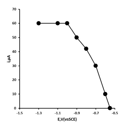
**Figure 3.** Effect of accumulation potential for a  $0.1 \text{ mM Pb}^{2+}$  solution in 0.3 M acetic acid containing 0.25 M KCl. Voltammetric conditions: Linear sweep stripping voltammetry, scan rate 50 mV/s; end potential 0.0 V.
