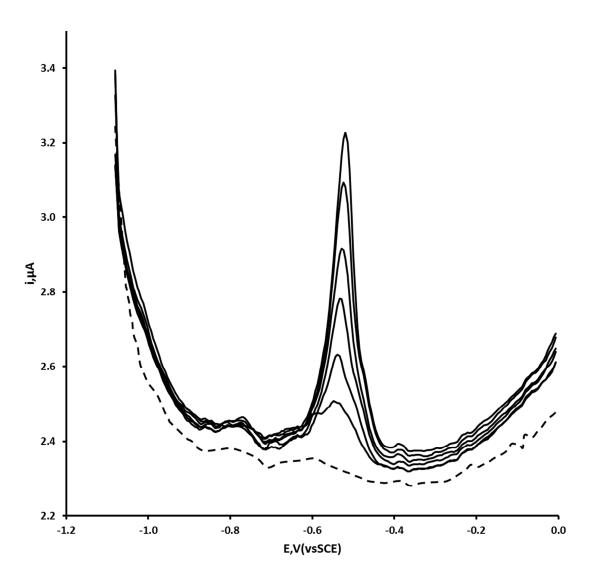
**Figure 7.** DPASVs of a representative drainage water sample spiked with 166 ng/mL Pb with added concentrations of Pb: 0 ng/mL; 83.0 ng/mL; 116 ng/mL; 249 ng/mL; 332 ng/mL; 415 ng/mL Pb added. Dashed line representative DPASV of unfortified drainage water sample. Accumulation time: 200 s, deposition potential: -1.1 V (vs. SCE).
