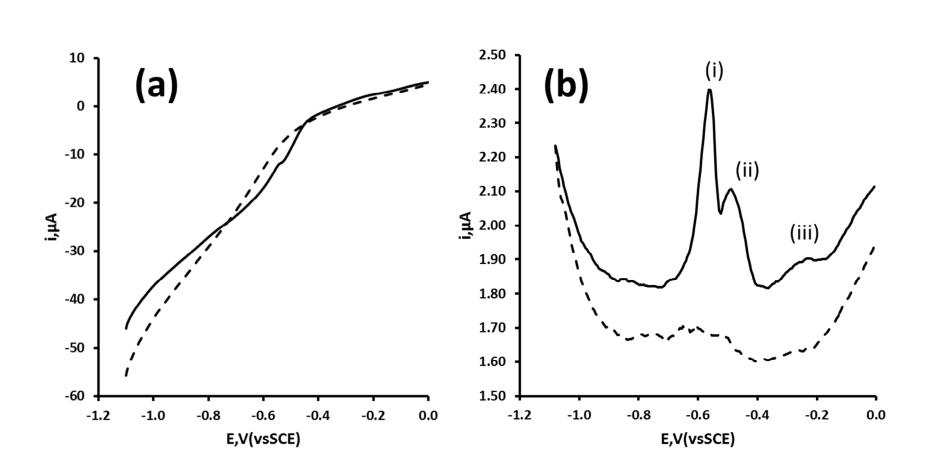
**Figure 4.** Effect of voltammetric waveform on the stripping voltammetric behaviour Pb. Solid line, in the presence of 415 ng/mL Pb and dashed line in the absence of Pb. (a) linear sweep (b) differential pulse voltammetry.
