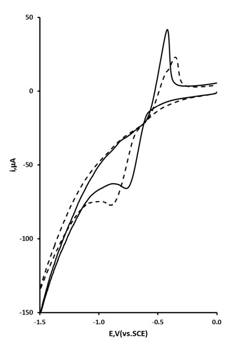
**Figure 2.** Cyclic voltammetric behaviour of 0.1 mM Pb at a drawn pencil in a 0.3 M acetic acid solution in the presence (solid line) of 0.25 M Cl and in the absence of Cl (dashed line). Voltammetric conditions: starting and end potential 0.0 V; switching potential -1.5 V; scan rate 50 mV/s.
