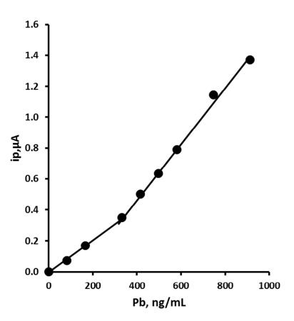
**Figure 6.** Calibration plot for Pb obtained by DPASV; supporting electrolyte 0.30 M acetic acid, 0.25 M KCl.
