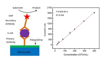
Detection of E. coli O157:H7 in beef juice with a detection limit of 19 CFU/mL. An assay time of 67 min was resulted due to the absence of sample pre-enrichment.
