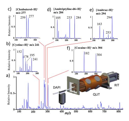
Figure 2. a) MS spectrum recorded by RIT for ions transferred from QLIT without mass selection. MS/MS spectra of protonated b) cysteine m/z 241, c) clenbuterol m/z 277, d) amitriptyline-d6 m/z 284, e) amitraz m/z 294 and f) cocaine m/z 304, precursor ions of each compounds mass selectively transferred from QLIT to RIT, fragmented in RIT, and MS analyzed. AC excitation of 80 mV and 169 kHz, q = 0.45 in QLIT;  $q = \sim 0.2$  for the trapping the ions in RIT,  $q = \sim 0.2$  for CID in RIT.
