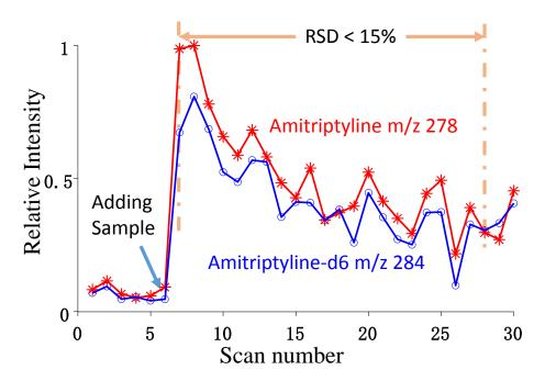
Figure 4. The signal intensities measure by RIT for sequentially mass-selectively transferred amitriptyline m/z 278 and amitriptyline-d6, m/z 284. Paper spray of methanol solution with amitriptyline and amitriptyline-d6 at 120 ng/mL, spray voltage of 4.3 kV. AC excitation of 80 mV 169 kHz, q=0.45, for mass-selective transfer from QLIT. q=0.2 for the trapping the ions in RIT.
