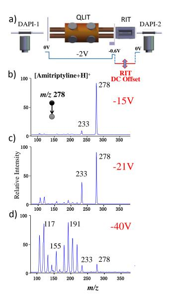
Figure 3. a) Instrument setup for MS/MS with CID during mass selective ion transfer. MS/MS spectra recorded for mass-selective transfer of protonated amitriptyline m/z 278 at RIT DC offset at b) -15V, c) -21V and d) -40V. AC excitation for axial ejection from QLIT, 80 mV and 169 kHz, q = 0.45 in QLIT; q = 0.2 for trapping the ions in RIT.
