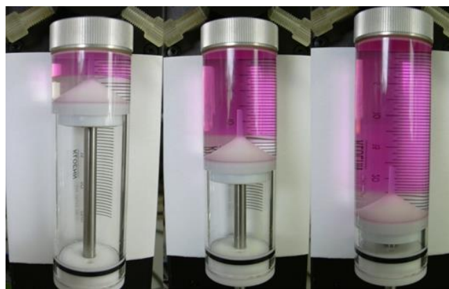
Figure 2. Syringe performance at 200 steps per second. The bottom layer is the dense acid brine solution, R1. The upper layer is seawater dyed for demonstration purposes. Photographs were obtained at 1, 2.5 and 4 minutes.
