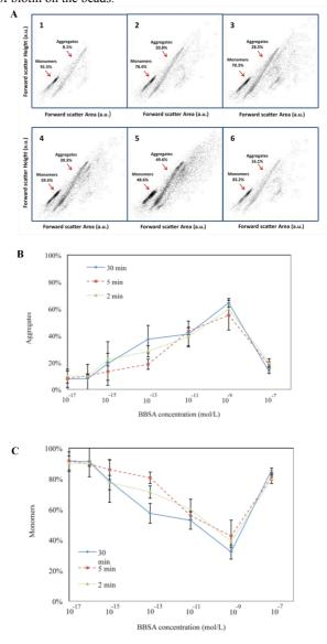
**Figure 2.** Results of the MBA assay for the detection of BBSA. **A.** Flow cytometry analysis of BBSA-streptavidin bead assays: (1) blank and (2) BBSA in the concentration of 3 x  $10^{-15}$ , (3) 3 x  $10^{-13}$ , (4) 3 x  $10^{-11}$ , (5) 3 x  $10^{-9}$ , and (6) 3 x  $10^{-7}$  M. **B** Proportion
