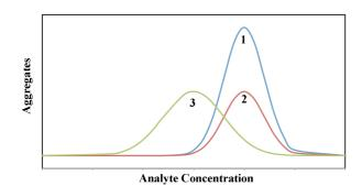
**Figure 3.** MBA assay response resulting from the change in the <sup>20</sup> physical and chemical properties of the SPM beads. (1) Reference binding curve, (2) decrease in ligand density on the beads, and (3) decrease in the number of beads used in the assay.
