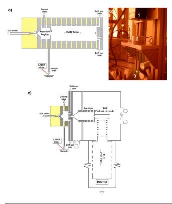
Figure 1. a) The schematic view of CD-IMS instrument, b) photograph with of the LD unit 1-LDM, 2-focusing lens, 3investigated surface, c) schematic view of APCDI-MS instrument.
