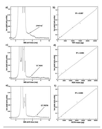
Figure 3 Measured sensitivities for a) 86 pg of TNT, c) 305 pg of RDX, e) 1.22 ng of PETN and investigated linear dynamic range of b) TNT, d) RDX and f) PETN.
