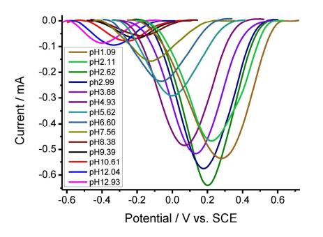
Fig 5. Quinone reduction peaks in square wave (SWV). Reduction peaks were obtained in different media (HCl/KCl buffer, citrate buffer, phosphate buffer, carbonate buffer and NaOH buffer solutions) at 0.01 M, ranging in pH from 2.11 to 12.93, 0.1 M HCl/KCl buffer at pH 1.09. SWV performed under optimised conditions: frequency – 150 Hz, step potential – 2 mV, amplitude – 200 mV 182x127mm (300 x 300 DPI)
