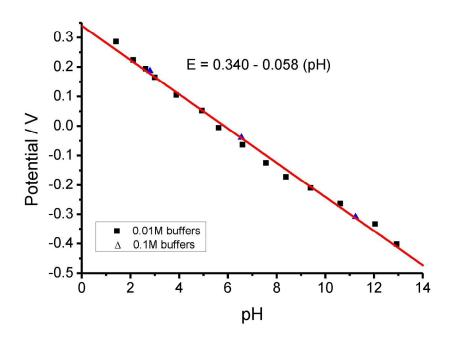
Figure 11. Calibration plot of the original reduction points in 0.01 M buffer solutions (black triangles), with reduction points of 0.1 M buffer solutions (blue triangles) added for comparison 182x127mm (300 x 300 DPI)
