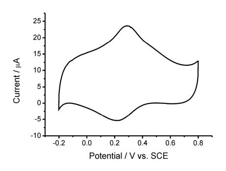
Fig 3. Typical CV of EPPG in 0.01 M HNO $_3$  + 100 mM KCl supporting electrolyte, from which surface coverage of quinone groups can be calculated 182x127mm (300 x 300 DPI)
