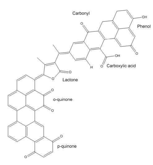
Fig 2. Representation of various functional groups present on graphitic carbon surfaces, adapted from reference [25] 152x148mm (300 x 300 DPI)
