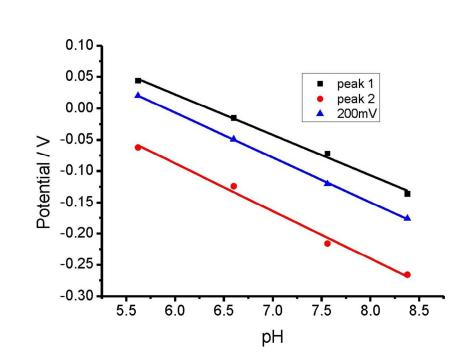
Figure 8. Calibration plot showing both peak 1 and peak 2 of the double peak reduction in 0.01 M phosphate buffer with amplitude 20 mV. Calibration for the reductions performed at 200 mV are shown as blue triangles, intermediate of the 2 peaks at 20 mV amplitude 115x80mm (300 x 300 DPI)
