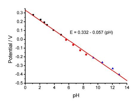
Fig 6. Calibration plot of SWV peak potential against pH for an EPPG in 0.01 M buffer solutions (with 0.1M HCI/KCI buffer solution at pH 1.09), showing a linear response with gradient of 57.0 mV / pH corresponding to a Nernstian behaviour. Black squares: low pH range, red circles: neutral pH range, blue squares: high pH range
