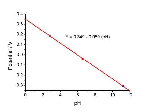
Figure 10. Calibration plot of the reduction peaks in 0.1 M buffer solutions. Back square corresponds to citrate buffer, red circle corresponds to phosphate buffer and blue triangle corresponds to carbonate buffer  $170 \times 119 \text{ mm}$  (300 x 300 DPI)
