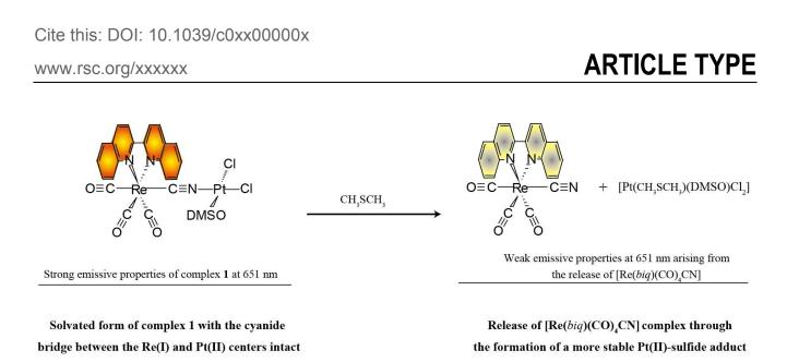
Figure 3. Proposed molecular recognition and luminescence signaling mechanism of complex 1 toward CH<sub>3</sub>SCH<sub>3</sub>.
