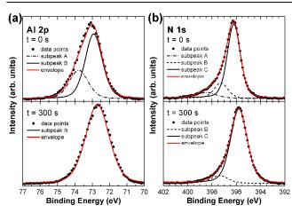
**Fig. 6** (a) Al 2p, and (b) N 1 s HR-XPS scans of 59.2-nm-thick AlN thin film deposited on Si (100) substrate using optimized HCPA-ALD parameters.
