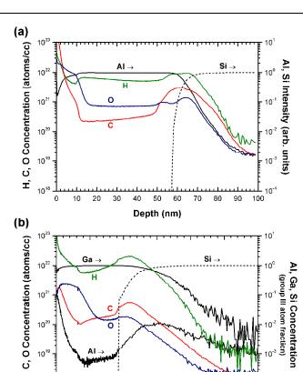
**Fig. 1** Impurity concentrations determined by SIMS depth profiling for 55 (a) AlN, and (b) GaN thin films deposited using NH<sub>3</sub> plasma. Silicon is not quantified in the layers, only plotted as the substrate layer marker.
