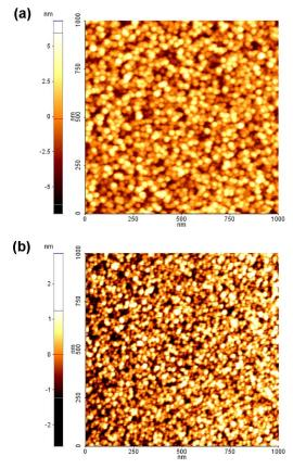
20 Fig. 9 Surface morphologies of (a) 59.2-nm-thick AlN, and (b) 20.1-nmthick GaN thin films deposited on Si (100) substrates using optimized HCPA-ALD parameters.
