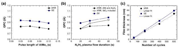
5 Fig. 4 (a) AlMe<sub>3</sub>, and (b) N<sub>2</sub>/H<sub>2</sub> saturation curves at 200 °C. For the AlMe<sub>3</sub> saturation curve, N<sub>2</sub>/H<sub>2</sub> flow rate and flow duration were kept constant at 50 + 50 sccm and 40 s, respectively. AlMe<sub>3</sub> pulse length was 0.06 s for the N<sub>2</sub>/H<sub>2</sub> saturation curve. (c) AlN film thickness plotted as a function of number of deposition cycles.
