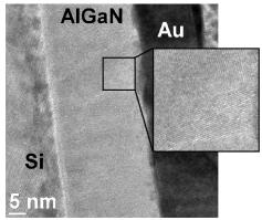
55 Fig. 12 Cross-sectional (a) bright-field STEM, and (b) HR-TEM images of 25.4-nm-thick Al<sub>0.68</sub>Ga<sub>0.32</sub>N thin film deposited on Si (111) substrate using N2/H2 plasma.
