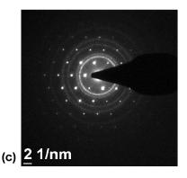
Fig. 3 Cross-sectional (a) TEM, and (b) HR-TEM images of 21-nm-thick GaN thin film deposited on Si (100) substrate using NH<sub>3</sub> plasma. FIB-induced SiO<sub>2</sub> damage layer formed at the GaN/Si interface during TEM sample preparation. (c) SAED pattern of the same sample.
