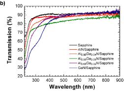
Fig. 13 (a) Spectral refractive indices, and (b) optical transmission spectra 60 of AlN, GaN, and Al<sub>x</sub>Ga<sub>1-x</sub>N thin films deposited Si (100) and double side polished c-plane sapphire substrates, respectively.
