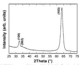
**Fig. 8** GIXRD pattern of 20.1-nm-thick GaN thin film deposited on *c*-plane sapphire substrate using optimized HCPA-ALD parameters.
