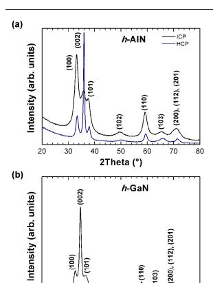
**Fig. 2** GIXRD patterns of (a) AlN, and (b) GaN thin films deposited on Si(100) substrates using NH<sub>3</sub> plasma. GIXRD pattern of the AlN thin film deposited using quartz-based ICP source<sup>21</sup> is also shown in (a) for 5 comparison.
