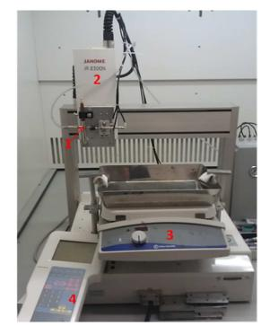
**Fig. 1** Spray set up of the Janome JR 2300N automatic robot showing; 1: airbrush with compressed air feed attached 2: mechanical robot with pneumatic arm 3: hot plate where substrate is placed and 4: programmable controller.
