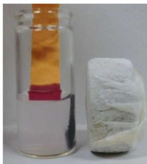
**Fig. 4.** The behaviour of Co@SiO<sub>2</sub> exposed to a magnet (right-side) after immersion in 1 M HCl. Particles in the sample bottle were attracted to the magnet. The photograph also shows that the color of the pH indicator paper turned from yellow to red in the acid solution.
