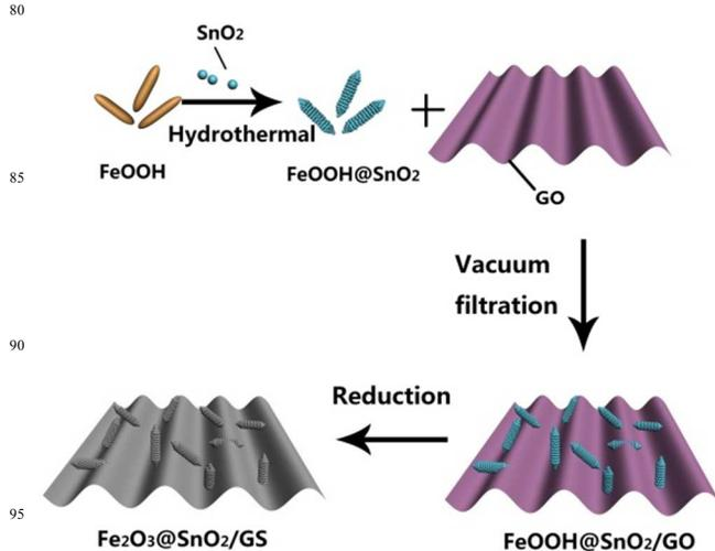
**Scheme 1** Schematic illustration of the synthesis process of Fe<sub>2</sub>O<sub>3</sub>@SnO<sub>2</sub>/GS film.
