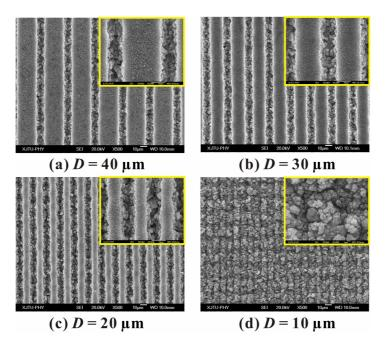
Figure 1. SEM images of various femtosecond-laser-induced line-patterned surfaces with different period (*D*): (a)  $D = 40 \mu \text{m}$ ; (b)  $D = 30 \mu \text{m}$ ; (c)  $D = 20 \mu \text{m}$ ; (d)  $D = 10 \mu \text{m}$ . The insets are corresponding magnified SEM images.
