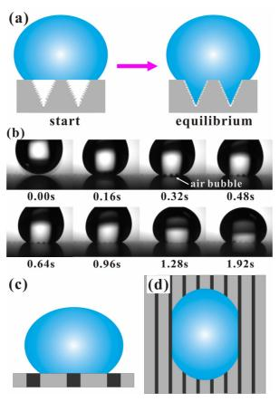
Figure 10. The underlying reasons for anisotropic wetting. (a) Schematic illustration of water droplet partly diving
