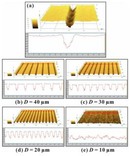
**Figure 2**. 3D and cross-sectional profiles of the femtosecond-laser-induced line-patterned surfaces. (a) A single microgroove fabricated by femtosecond laser scanning at laser power of 30 mW and speed of 4 mm/s. (b-e) the as-prepared line-patterned surfaces with different period (*D*): (b)  $D = 40 \mu m$ ; (c)  $D = 30 \mu m$ ; (d)  $D = 20 \mu m$ ; (e)  $D = 10 \mu m$ .
