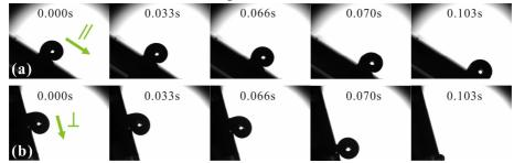
Figure 7. Time sequences of snapshots of a water droplet rolling on the as-prepared surface with D of 25  $\mu$ m along the parallel and perpendicular directions. The as-prepared surface in (a) and (b) is tilted 31° and 76°, respectively.
