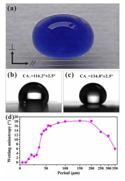
**Figure 9**. Anisotropic wetting of the line-patterned surfaces. (a) Optical micrograph of a blue-colored water droplet on the patterned as-prepared surface, revealing an elongated shape. (b,c) Images of water droplet shape for the parallel (b) and perpendicular (c) directions. (d) The wetting anisotropy as a function against the period (*D*) of microgroove arrays.
