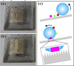
Figure 5. Self-cleaning effect of the as-prepared superhydrophobic surface with *D* of 10 μm. (a) Graphite power spreading on the surface. (b) A water droplet rolling through the surface. (c) Schematic depicting the motion of a liquid droplet on an inclined superhydrophobic substratum covered with "dirt".
