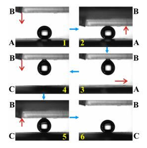
**Figure 6.** Transfer process of a 7 μl water droplet from the A-surface to C-surface using the B-surface. Surfaces of A, B, and C were as-prepared line-patterned surfaces with D of 10 μm, 30 μm, and 20 μm, respectively.
