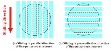
**Figure 8**. Schematic illustration of the three-phase contact line from the top view (cyan, flat PDMS parts; white, microgroove parts; circle, contact part of water and solid surface).
