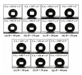
Figure 4. Images of water droplet shape in two views (perpendicular  $(CA_{\perp})$  to and parallel  $(CA_{\parallel})$  to the direction
