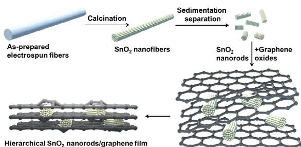
**Fig. 1.** Schematic illustration of the preparation of the hierarchical SnO<sub>2</sub> nanorod/graphene film.
