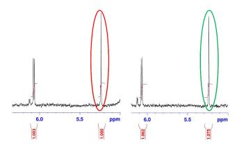
**Figure 1** <sup>1</sup>H NMR spectra of **2***R* incubated with AMACR, showing αproton at *ca.* 5.3 p.p.m. Left panel, heat-inactivated enzyme; Right panel, live enzyme, showing no reduction in signal.
