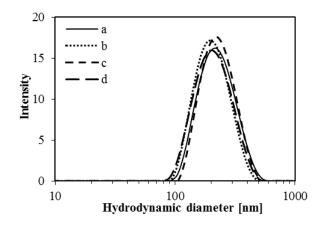
**Figure 5.** Hydrodynamic diameters determined for hydrothermally treated MSNs at different stages of the functionalization process; a) native particles, b) amino-functionalized particles, and c-d) DFO-functionalized particles. The particle concentration was 100  $\mu$ g/ml in all cases and the measurements a)-c) were carried out in a 100 mM KCl solution at pH 7, d) was measured in cell culture media with 10 % FCS.
