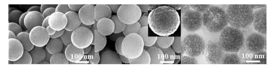
**Figure 3.** SEM images of non-expanded (left) and pore-expanded (in the middle) MSNs including a close-up view of a particle and a related TEM image (right).
