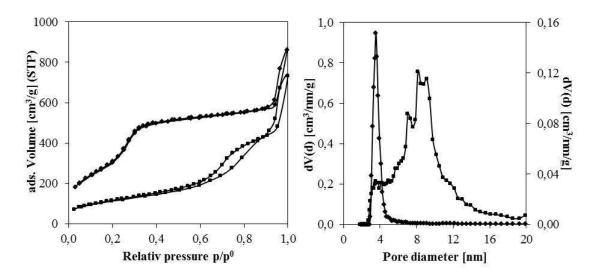
**Figure 2.** Nitrogen adsorption-desorption isotherms (left) and pore size distribution (right) of original MSN ( $\blacklozenge$ ) and pore-expanded MSN ( $\blacksquare$ ) samples.
