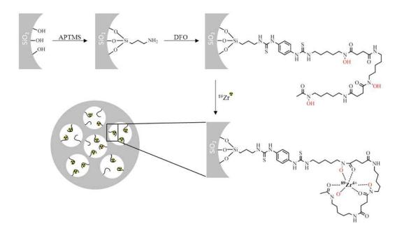
**Figure 1.** A schematic representation of MSNs functionalized with APTMS, coupled with DFO and radiolabeled with radionuclide <sup>89</sup>Zr.
