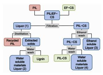
Scheme 2 Lignin-extraction process for CS using a PIL with labelled process streams.
