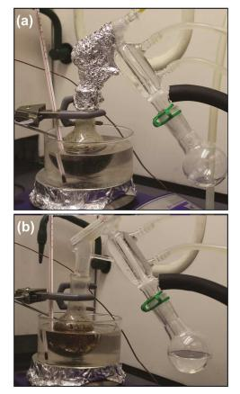
Fig. 3 Distillation apparatus used to separate the PILs from lignin showing: (a) initial setup and (b) after completed collection of the distillate (PIL).
