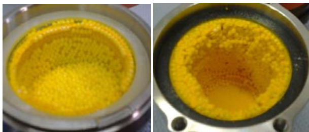
Figure 3 Hindered milling ball movement by enclosure of the milling balls in the substrate-product mixture. Reaction conditions: P7-45-20, rpm = 1000 \text{ min}^{-1} , d_{MB} = 2 \text{ mm} , \Phi_{MB,packing} = 0.46 .
