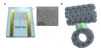
Figure 1| Network of single-walled carbon nanotubes (SWNTs) and the bonding of a lanthanide atom at a SWNT junction. a, SWNT film mounted on gold contacts for e-beam deposition of lanthanides; inset shows an SEM image of SWNT film. b, schematic of two SWNTs bridged by a lanthanide atom.
