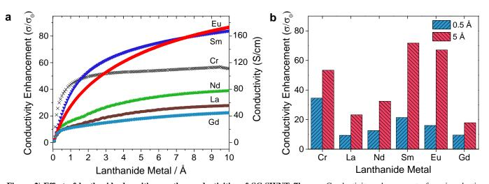
Figure 2| Effect of lanthanide deposition on the conductivities of SC-SWNT films. a, Conductivity enhancement of semiconducting single-walled carbon nanotube (SC-SWNT) films of thickness, t = 8nm, as a function of metal deposition. b, Conductivity enhancement of SC-SWNT films after the deposition of 0.5 Å and 5 Å of lanthanide metal.
