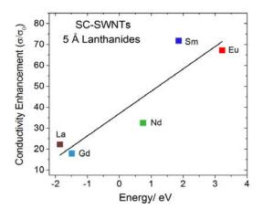
Figure 3| Enhancement of carbon nanotube conductivity as a function of the 4f<sup>n</sup> 6s<sup>2</sup>  $\rightarrow$  4f<sup>n-1</sup> 5d<sup>1</sup> 6s<sup>2</sup> transition energies of the lanthanides. Conductivity enhancement of SC-SWNT films of 8 nm thickness after deposition of 5 Å La, Gd, Nd, Sm and Eu; the conductivity values are given relative to the initial conductivity ( $\sigma_0$ ) of the pristine SC-SWNT film.
