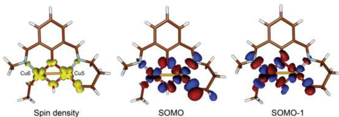
Figure 7. Spin density map and SOMOs of a dinuclear Cu5-Cu6 unit of complex 1 computed at the M06-2X/6-31+G* level of theory.
