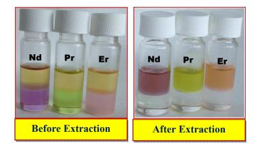
Rare earths can be extracted from molten calcium nitrate tetrahydrate to the ionic liquid tricaprylmethylammonium nitrate at very high loading concentrations.
