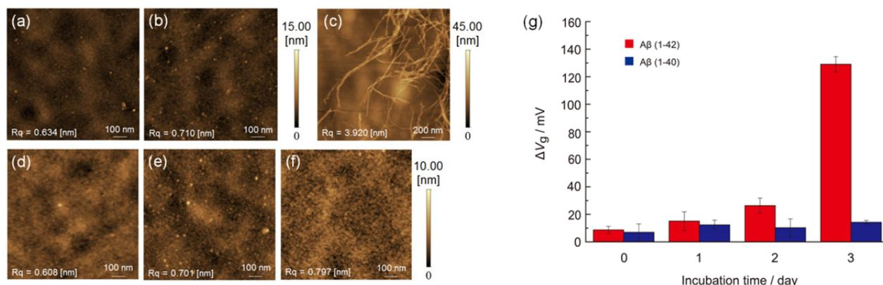
Figure 2. Comparison of Amyloid growth between A $\beta$ 42 and A $\beta$ 40. Atomic force microscopy images of surfaces of the assay device treated with (a–c) A $\beta$ 42 and (d–f) A $\beta$ 40. The incubation duration of the amyloid were (a, d) 1 day, (b, e) 2 days, and (c, f) 3 days, respectively. (g) Relation between incubation time and the sensor responses caused by A $\beta$  adsorption for the assay devices.
