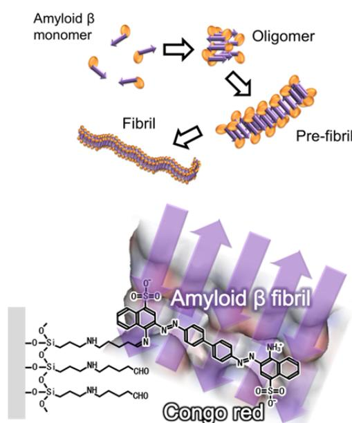
Figure 1. Schematic illustration of the label-free electrical assay for discriminating fibrous A $\beta$  proteins. The assay detects intrinsic charges of fibrous A $\beta$  proteins, which possess the interaction with Congo red molecules immobilized on the sensing surface.
