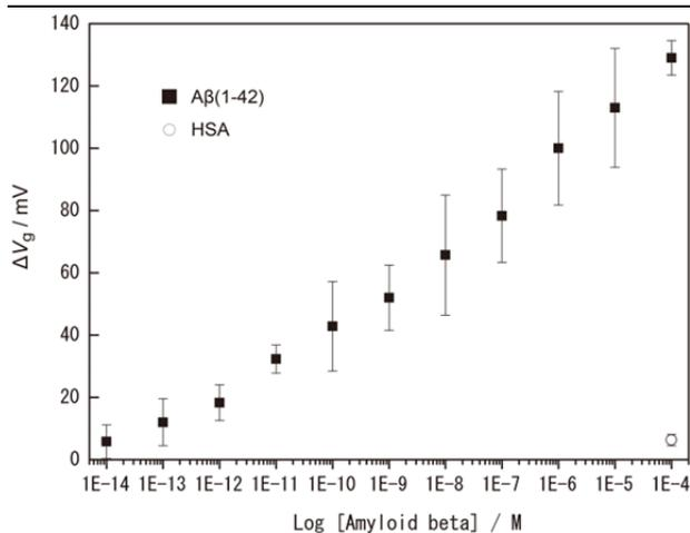
Figure 3. Quantitative determination of fibrous Aβ<sub>42</sub> (incubated for 3 days) (closed symbols) ranging from 10 fM to 100 μM using the FET-based assay. The open symbol indicates the sensor response for non-related protein (HSA, 100 μM).
