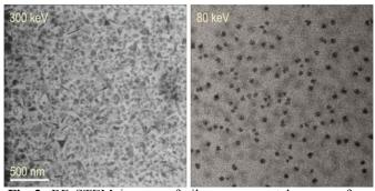
**Fig 2.** BF STEM images of silver nanocrystals grown from solution at 300 kV (left) and 80 kV (right). The magnification was M=40000X, pixel-dwell time was 3  $\mu$ s, calibrated beam current 7.1 pA and image size was 1024x1024 pixels, which corresponded to an electron dose per frame of 39.1 e/nm<sup>2</sup>f.
