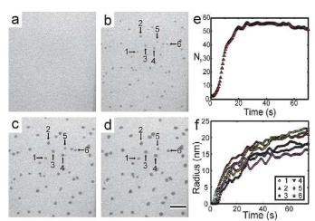
Fig 1. Time lapsed series of BF STEM images showing silver nanocrystal formation from a AgNO<sub>3</sub> precursor solution at t=0 s (a), t=15 s (b), t=45 s (c) and t=75 s (d), relative to the initial irradiation. Scale bar is 200 nm, the accelerating voltage was 200 kV and the beam current was  $i_e = 40$  pA. The total number of particles (e) and radius of particles 1-6 (f) as a function of time. Reprinted with permission. 4 Copyright 2012 American Chemical Society.
