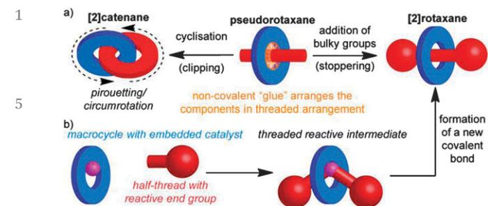
Fig. 1 Synthesis of rotaxanes and catenanes by (a) the passive and (b) the active template synthesis of a [2]rotaxane.
