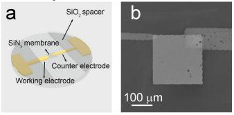
**Fig. 1** (a) Schematic of the  $SiN_x$  grid utilized for assembling the insitu environmental cell. (b) SEM image of the 50 nm  $SiN_x$  window patterned with gold electrodes, used in this study, imaged after testing.
