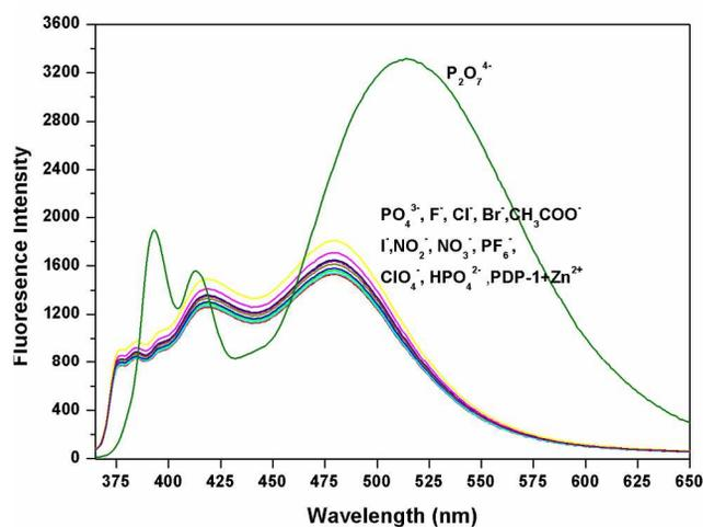
Figure-5: Fluorescence spectra of PDP-1+ $Zn^{2+}$  ( $1 \times 10^{-5} \text{ mol L}^{-1}$ ) in the presence of  $\text{PO}_4^{3-}$ ,  $\text{F}^-$ ,  $\text{Cl}^-$ ,  $\text{Br}^-$ ,  $\text{I}^-$ ,  $\text{NO}_3^-$ ,  $\text{PF}_6^-$ ,  $\text{ClO}_4^-$ ,  $\text{HPO}_4^{2-}$  and  $\text{P}_2\text{O}_7^{4-}$  (10  $\mu\text{M}$ ) in aqueous HEPES buffer (10 mM HEPES pH 7.4) containing  $\text{CH}_3\text{CN}-\text{H}_2\text{O}$  (30:70). Excitation was performed at 350 nm
