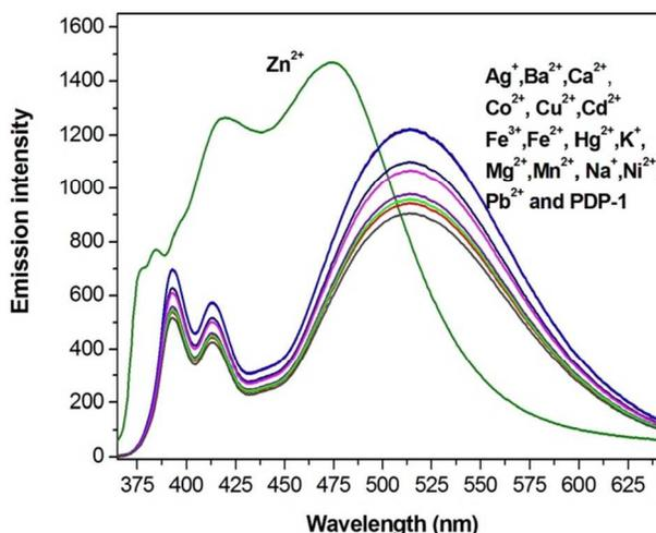
Figure-2: Fluorescence spectra of PDP-1 in the presence of  $Fe^{3+}$ ,  $Fe^{2+}$ ,  $Ag^+$ ,  $Ca^{2+}$ ,  $Cd^{2+}$ ,  $Co^{2+}$ ,  $Cu^{2+}$ ,  $Hg^{2+}$ ,  $K^+$ ,  $Mg^{2+}$ ,  $Mn^{2+}$ ,  $Na^+$ ,  $Ni^{2+}$ ,  $Pb^{2+}$  and  $Zn^{2+}$  (10  $\mu$ M) in aqueous HEPES buffer (10 mM HEPES pH 7.4) containing  $H_2O$ - $CH_3CN$  (30:70). Excitation was performed at 350 nm.
