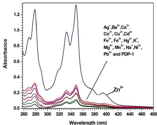
Figure-1: UV-vis absorption spectra of PDP-1 (10  $\mu$ M) in the presence of  $Fe^{3+}$ ,  $Fe^{2+}$ ,  $Ag^+$ ,  $Ca^{2+}$ ,  $Cd^{2+}$ ,  $Co^{2+}$ ,  $Cu^{2+}$ ,  $Hg^{2+}$ ,  $K^+$ ,  $Mg^{2+}$ ,  $Mn^{2+}$ ,  $Na^+$ ,  $Ni^{2+}$ ,  $Pb^{2+}$  and  $Zn^{2+}$  (10  $\mu$ M) in aqueous HEPES buffer (10 mM HEPES, pH=7.4,  $H_2O$ :  $CH_3CN$ = 30:70).
