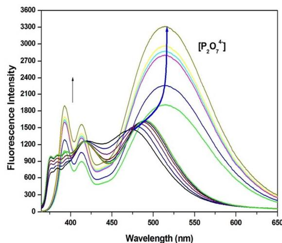
Figure-6: Fluorescence emission spectrum of PDP-1+ $Zn^{2+}$  ( $1 \times 10^{-5} \text{ mol L}^{-1}$ ) upon addition of pyrophosphate ions (0-100 equiv) in aqueous HEPES (10 mM HEPES, pH=7.4,  $\text{H}_2\text{O}:\text{CH}_3\text{CN}=30:70$ ).
