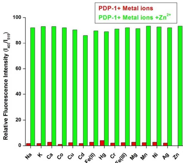
Figure-4: Fluorescence response ( $I/I_0$ ) of PDP-1 (10  $\mu\text{M}$ ) in  $\text{CH}_3\text{CN}/\text{H}_2\text{O}$  (30:70 v/v) to 10  $\mu\text{M}$  of various tested metal ions (green bar) and to the mixture of 10  $\mu\text{M}$  of tested metal ions with 10  $\mu\text{M}$   $Zn^{2+}$  ion (red bar).
