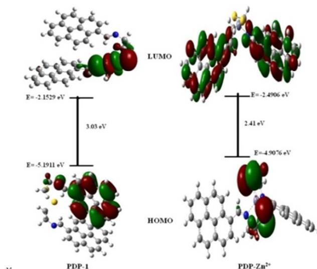
Figure-9: Frontier molecular orbital diagram of PDP-1 and PDP-1 + Zn<sup>2+</sup>
