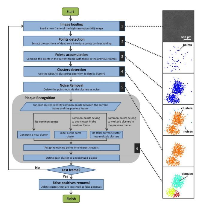
Figure 2. The plaque recognition algorithm structure.
