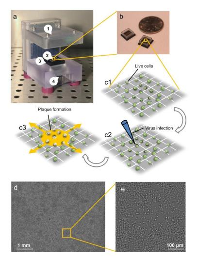
Figure 1. The ePetri device setup. (a) The ePetri device prototype. (b) Image sensor with reservoir. (c1-c3) Viral infection and plaque growth on the image sensor. (d) A representative, full field-of-view, high-resolution image with (e) a typical growing plaque zoomed in.
