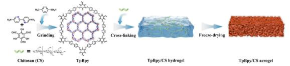
Scheme 1 Schematic diagram of the TpBpy/CS aerogel synthesis.
