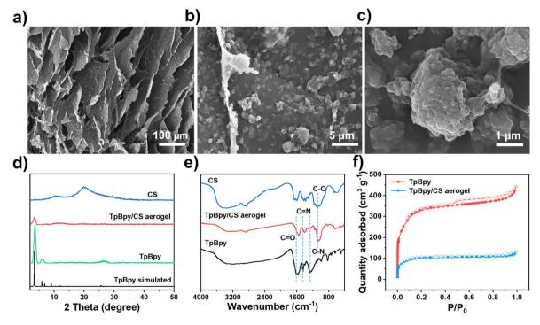
Fig. 1 (a–c) SEM micrographs of TpBpy/CS aerogel; (d) XRD patterns and (e) FT-IR spectra of CS, TpBpy, and TpBpy/CS aerogel; (f)  $N_2$  adsorption–desorption isotherms of TpBpy/CS aerogel and TpBpy.
