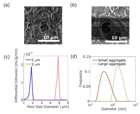
Fig. 1 SEM images of silica monolithic columns with pore size distribution peaks at 2 μm (a) and 5 μm (b). (c) Pore size distributions of silica monolithic columns with pore size: the peak at 2 µm (solid blue line) and 5 µm (dashed red line). (d) Histogram of DLS of small aggregates with a diameter distribution peak at 40 nm (solid orange line) and large aggregates with a diameter distribution peak at 171 nm (dashed green line).
