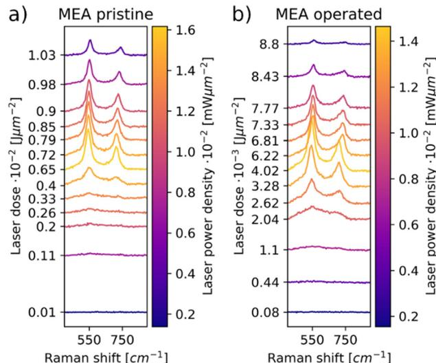
Fig. 4 Laser power series performed on the anode of the pristine (a) and operated MEA (b) samples. Amorphous  $\text{IrO}_x$  signal is observable at the lower laser powers, indicating some degree of pre-oxidation. This pre-oxidation is more pronounced in the spectra of the operated sample.
