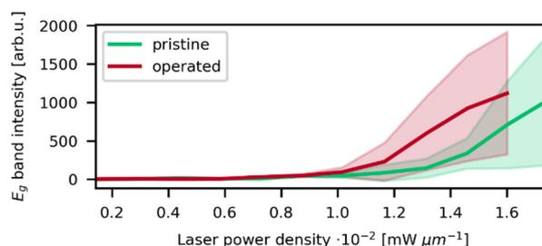
Fig. 5 Intensity of the  $E_g$  band vs. laser power density from the laser power series of the pristine and operated anodes. Standard deviation of the intensity is depicted as the filled area around the plot. An oxidation onset at lower laser power density is observable for the operated sample.
