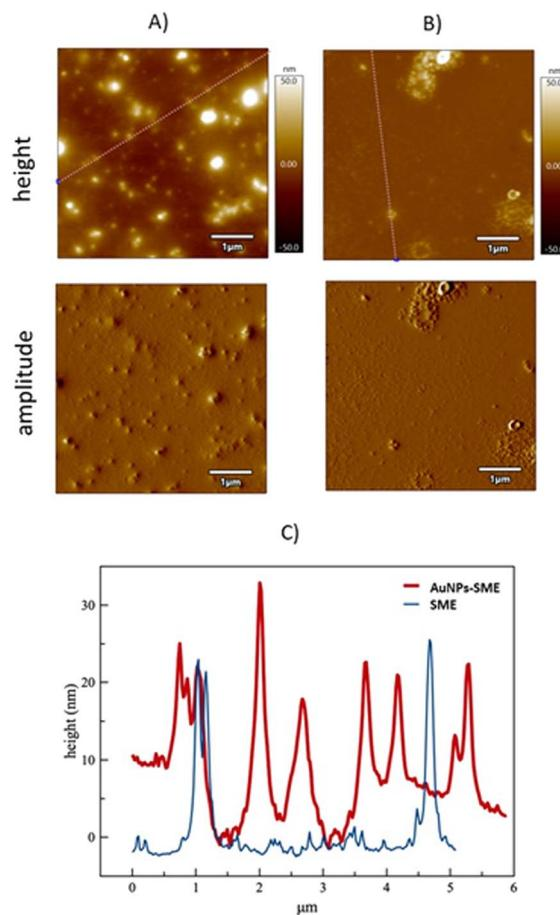
Fig. 2 AFM images: height and amplitude images ( $5\text{ }\mu\text{m} \times 5\text{ }\mu\text{m}$  scan size) of AuNPs-SME (A) and SME (B) samples. In (C) the comparison of the section analysis (dashed lines in the height micrographs) for the two samples.
