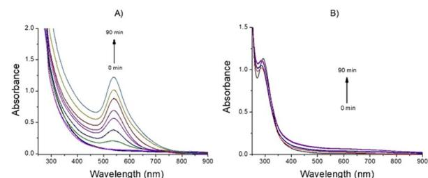
Fig. 3 Optical absorption changes at various reaction times (0, 10 min, 20 min, 30 min 40 min, 50 min, 60 min, 70 min, 80 min and 90 min) and at  $70\text{ }^\circ\text{C}$  for the AuNPs-SME process formation (A) and for the blank-reaction without SME (B).
