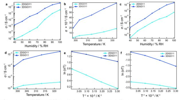
Fig. 3 OH<sup>-</sup> conductivities of 2DGO11 and 3DGO11: humidity dependent OH<sup>-</sup> conductivity in the (a) in-plane and (c) through-plane direction measured maintaining several humidified conditions at 25 °C; temperature-dependent OH- conductivity in the (b) in-plane and (d) through-plane direction measured at different temperatures under 90% RH; Arrhenius plots of  $\ln(\sigma T)$  vs.  $T^{-1}$  for (e) in-plane pathways and (f) the through-plane route evaluated at 90% RH.
