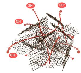
$\begin{tabular}{lll} Scheme 1 & OH^- & ion conductivity using three-dimensional alkaline graphene oxide. \\ \end{tabular}$
