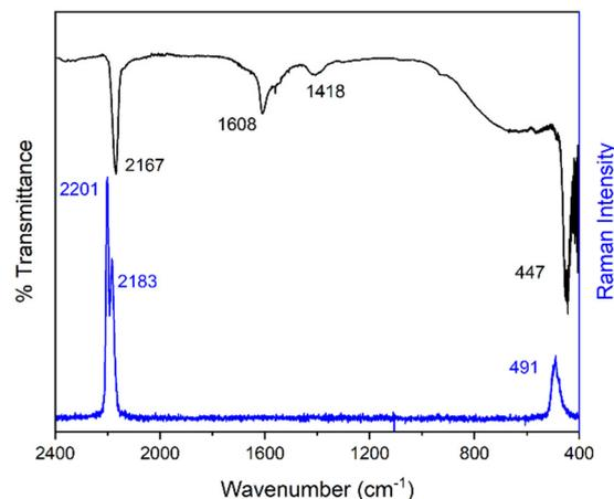
Fig. 6 Raman and infrared spectra of Co-PBA.
