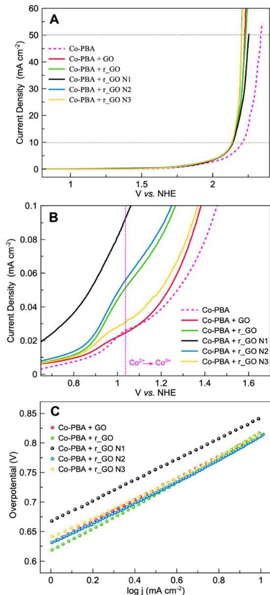
Fig. 8 Electrochemical experiments of the hybrid composites performed in  $0.5 \text{ mol L}^{-1} \text{ KNO}_3$  at a scan rate of  $5 \text{ mV s}^{-1}$ . (A) Linear sweep voltammetry (LSV), (B) the redox process  $\text{Co}^{2+}/\text{Co}^{3+}$  and (C) the Tafel plot.
