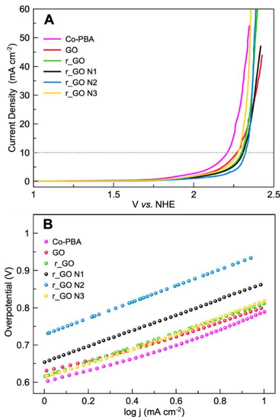
Fig. 7 Electrochemical experiments of Co-PBA and graphene-based materials performed in 0.5 mol L<sup>-1</sup> KNO<sub>3</sub> at a scan rate of 5 mV s<sup>-1</sup>. (A) Linear sweep voltammetry (LSV) and (B) Tafel plot.
