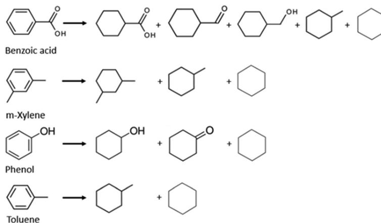
Fig. 15 Main components from plastic pyrolysis oil and the possible products from ECH.
