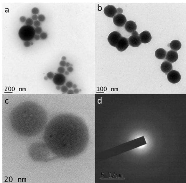
Fig. 9 TEM analysis of the CD-SiO<sub>2</sub> 1:0.25 nanocomposite (a–c) at different magnifications and (d) SAED pattern.
