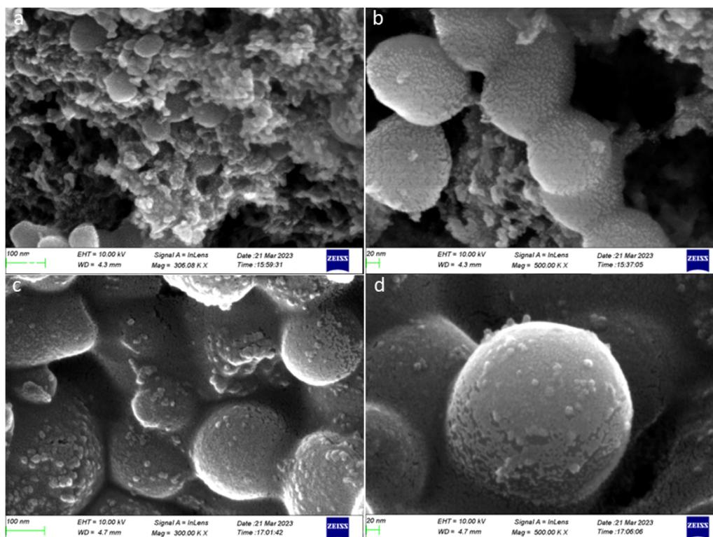
Fig. 8 FE-SEM analysis of (a and b) CD-SiO<sub>2</sub> 1:0.1 nanocomposite and (c and d) CD-SiO<sub>2</sub> 1:0.25 nanocomposite.
