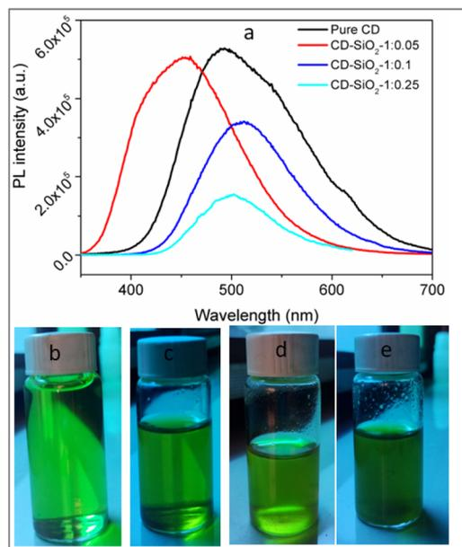
Fig. 6 (a) Photoluminescence spectra of carbon dots and carbon dot embedded silica nanocomposites recorded at an excitation wavelength of 320 nm and (b–e) photographs showing the emission behaviour of carbon dots and carbon dot embedded silica nanocomposites under UV light.
