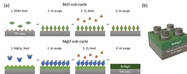
Fig. 1 Schematic representation of (a) the super-cycle ALD technique used for BMO film deposition. The BMO composition is controlled by adjusting the BeO and MgO sub-cycle ratios. (b) Illustration of the MIM-structured device, designed to assess the electrical performance of the fabricated films.
