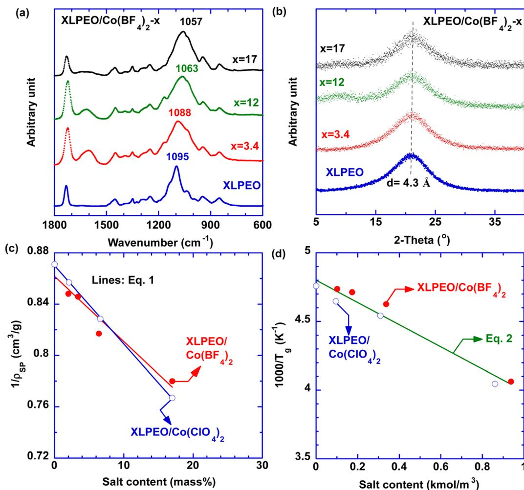
Fig. 2 Physical properties of SPNs. (a) FTIR spectra and (b) XRD patterns of XLPEO/ $\text{Co}(\text{BF}_4)_2$ . (c) Correlation between  $\rho_{\text{SP}}$  and the salt content using eqn (1). (d) Correlation between  $T_g$  and the salt content using eqn (2).
