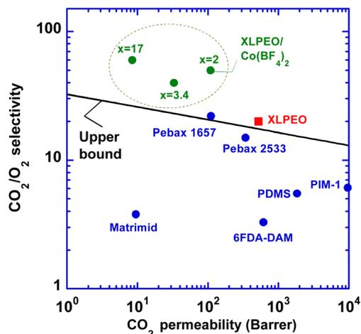
Fig. 5 Superior  $\text{CO}_2/\text{O}_2$  separation properties in  $\text{XLPEO}/\text{Co}(\text{BF}_4)_2$  ( $x = 2, 3.4, \text{ and } 17$ ) compared with Robeson's upper bound,<sup>36,37</sup> and representative polymers, including Matrimid,<sup>6</sup> Pebax 1657 and 2533,<sup>9</sup> 6FDA-DAM,<sup>38</sup> PDMS,<sup>1</sup> and PIM-1.<sup>39</sup>
