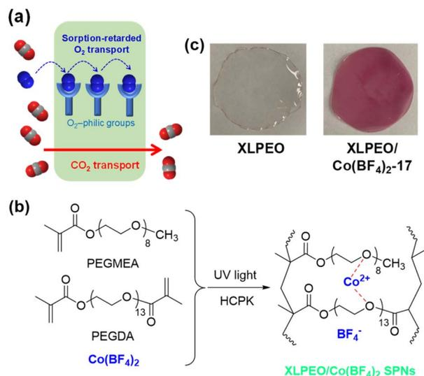
Fig. 1 Co<sup>2+</sup>-coordinated SPNs with superior CO<sub>2</sub>/O<sub>2</sub> separation properties. (a) Schematic of O<sub>2</sub>-retarded transport facilitating CO<sub>2</sub>/O<sub>2</sub> separation. (b) Schematic of XLPEO prepared from PEGDA and PEGMEA and its interactions with Co(BF<sub>4</sub>)<sub>2</sub>. (c) Photos of XLPEO/salt films.
