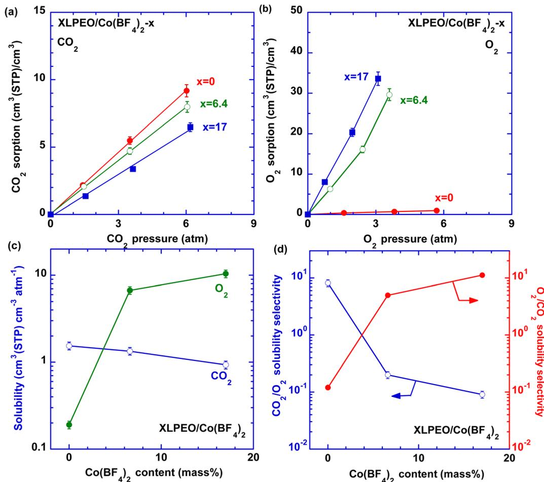
Fig. 3 Enormous O<sub>2</sub> sorption in XLPEO/Co(BF<sub>4</sub>)<sub>2</sub> SPNs at 35 °C. Effect of the Co(BF<sub>4</sub>)<sub>2</sub> loading on (a) CO<sub>2</sub> sorption isotherms, (b) O<sub>2</sub> sorption isotherms, (c) CO<sub>2</sub> and O<sub>2</sub> solubility, and (d) CO<sub>2</sub>/O<sub>2</sub> solubility selectivity.
