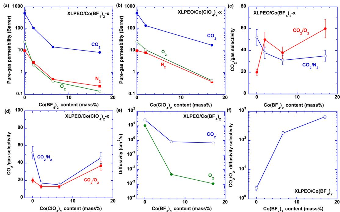
Fig. 4 Pure-gas transport properties of the SPNs at 35 °C. Dependence of gas permeability on (a)  $\text{Co}(\text{BF}_4)_2$  loading and (b)  $\text{Co}(\text{ClO}_4)_2$  loading. Dependence of  $\text{CO}_2/\text{gas}$  selectivity on (c)  $\text{Co}(\text{BF}_4)_2$  loading and (d)  $\text{Co}(\text{ClO}_4)_2$  loading. Effect of the  $\text{Co}(\text{BF}_4)_2$  loading on (e)  $\text{CO}_2$  and  $\text{O}_2$  diffusivity and (f)  $\text{CO}_2/\text{O}_2$  diffusivity selectivity.
