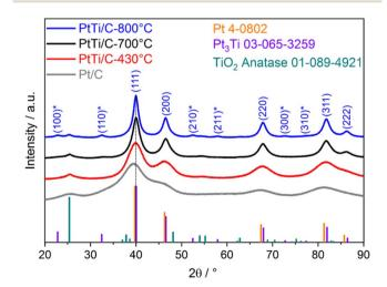
Fig. 2 XRD patterns of the three PtTi/C catalysts as a function of reductive annealing temperature. The reference diffraction patterns of the different crystal structures are displayed as colored bars at the bottom. The indices of the crystal planes correspond to the intermetallic  $Pt_3Ti$  phase, where \* denotes the superlattice planes. The dotted line at the (111) reflection illustrates the shift between the patterns.
