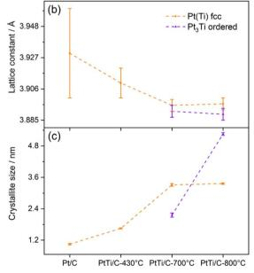
Fig. 3 Structural impact of annealing temperature as derived from Rietveld refinement: (a) phase composition with the graphite phase subtracted, (b) lattice constant and (c) crystallite size (LVol-B) of Pt(Ti) fcc (orange) and Pt<sub>T</sub>Ti (violet). Dashed lines are a guide to the eye.
