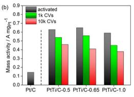
Fig. 6 (a) ECSA and (b) Pt mass activity of PtTi/C-0.5, -0.65 and -1.0 after 25 (black) for 1000 (green) and 10 000 (red) voltage cycles - values calculated from relative stabilities. Pt/C mass activity after 25 voltage cycles is given for comparison.
