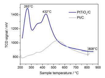
Fig. 1 Temperature-programmed reduction profiles of  $PtTiO_x/C$  and Pt/C recorded at a heating rate of 10 K min<sup>-1</sup> in 4 vol%  $H_2/Ar$ . TCD = thermal conductivity detector.
