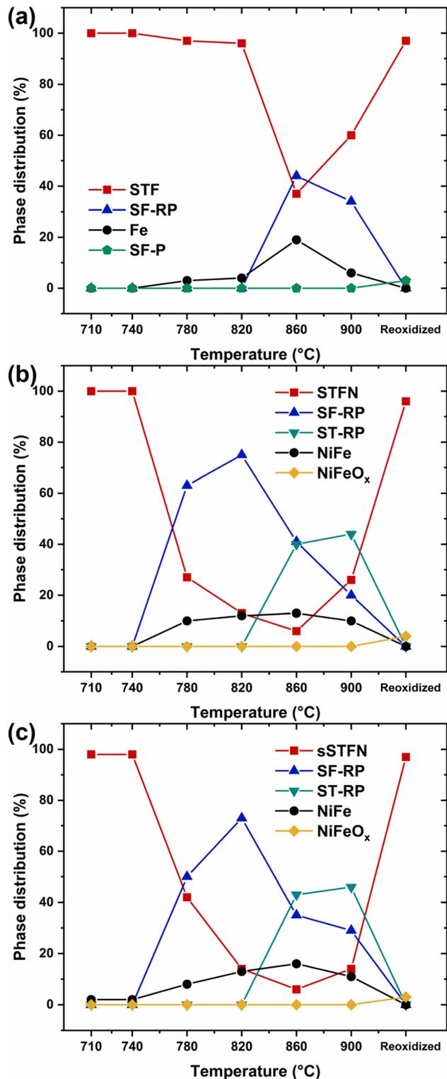
Fig. 7 Relative phase distribution for (a) STF, (b) STFN and (c) sSTFN reduced at temperatures of 710–900 °C in 50% Ar/50% H<sub>2</sub> for 8 h and reoxidized at 900 °C in air for 8 h.
