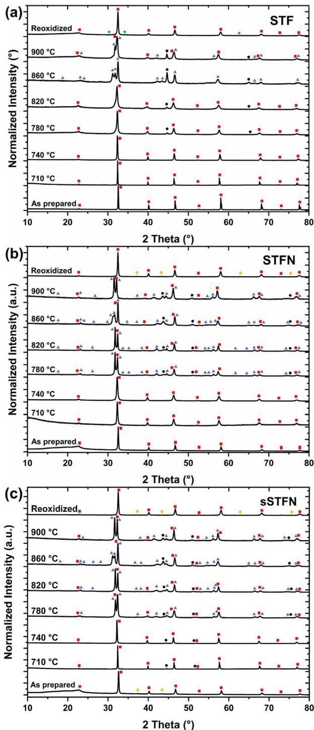
Fig. 6 Diffractograms for (a) STF, (b) STFN and (c) sSTFN in their as prepared, reduced (at 710–900 °C in Ar/50% H<sub>2</sub>) and reoxidized (at 900 °C for 3 h in air) state. Red squares denote the perovskite phase, blue triangles Ruddlesden–Popper phases, black circles metallic Fe/Ni phases, green pentagons denote a strontium ferrite perovskite phase, and yellow diamonds iron or nickel oxide phases.
