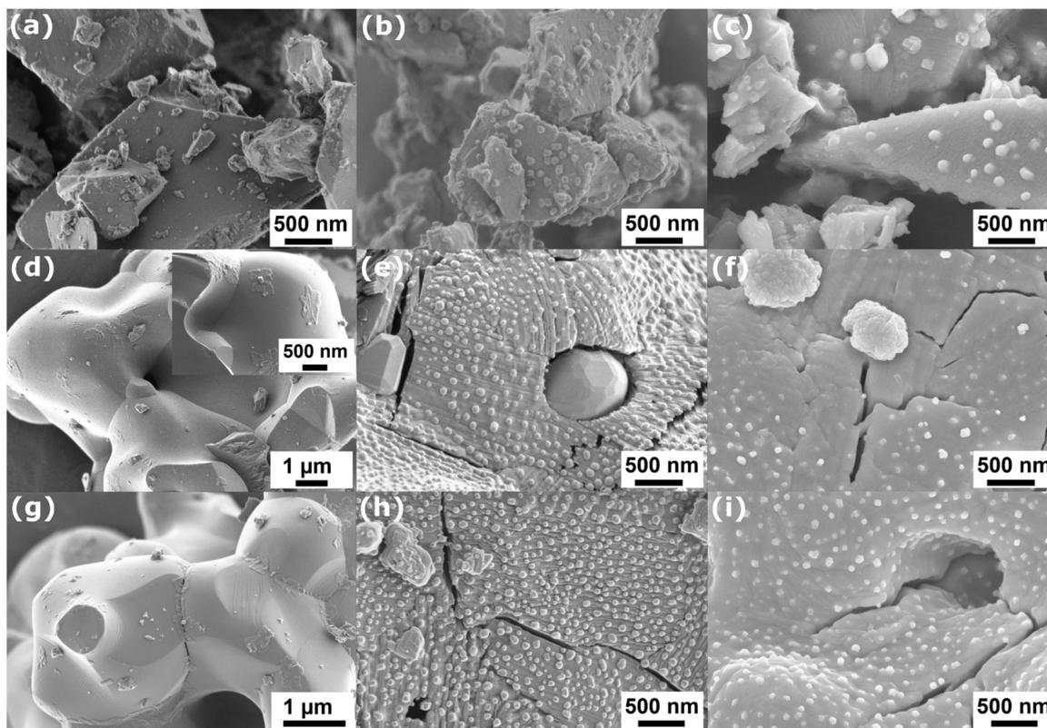
Fig. 2 SEM micrographs for STF, STFN and sSTFN in (a, d, g) as prepared, (b, e, h) reduced at 900 °C in 50% Ar/50% H<sub>2</sub> and (c, f, i) reoxidized state.
