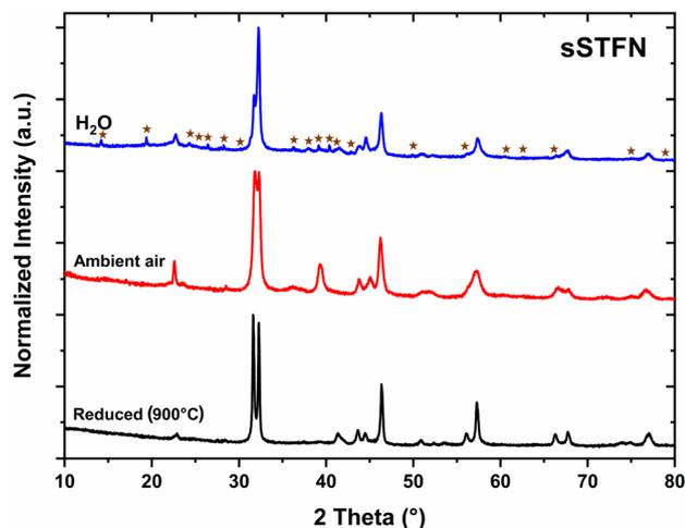
Fig. 8 Diffractograms for sSTFN recently reduced (at 900 °C in 50% Ar/50% H<sub>2</sub>), reduced and stored in ambient air for 4 weeks or immersed into H<sub>2</sub>O. Brown stars denote potential secondary phase reflexes (e.g., strontium hydroxides or iron(oxide)-hydroxides).
