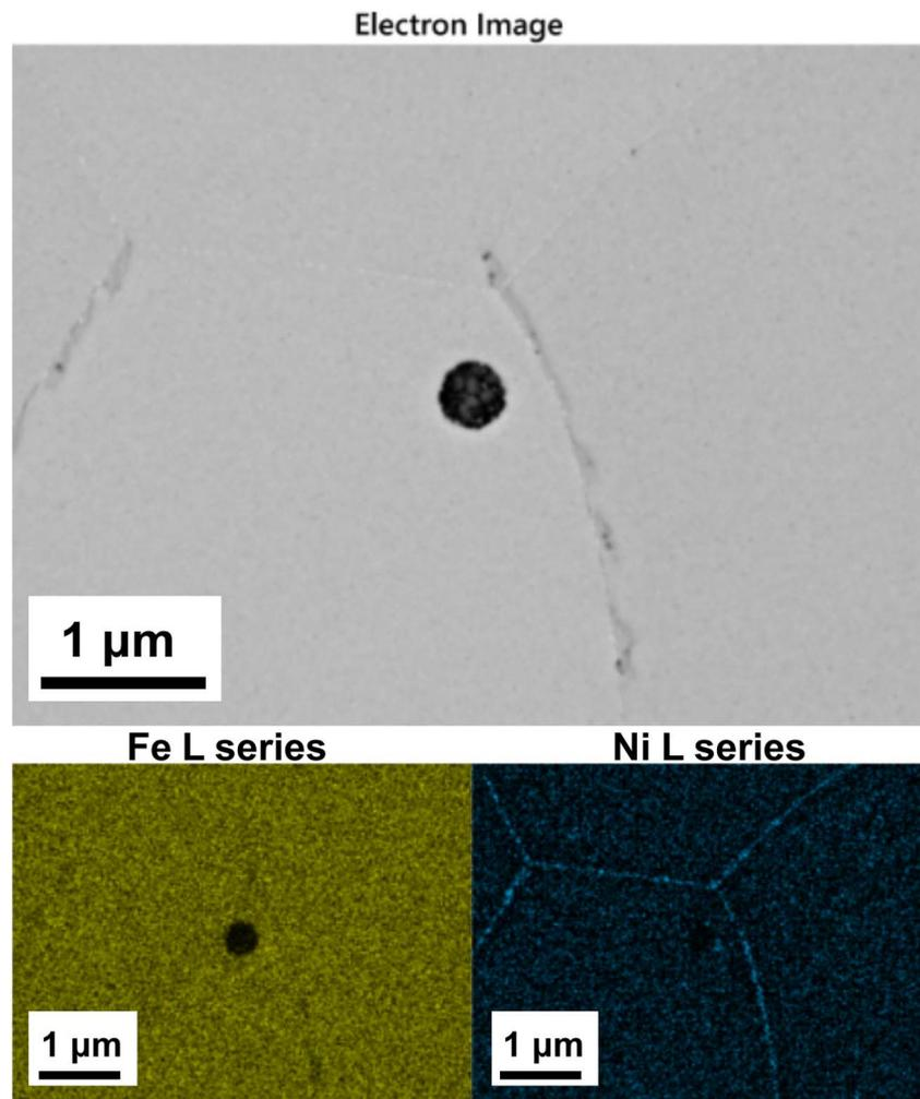
Fig. 4 EDS analysis of a cross-section of STFN reduced at 710 °C in 100% H<sub>2</sub>, analyzed with EDS (black spot belongs to a pore).
