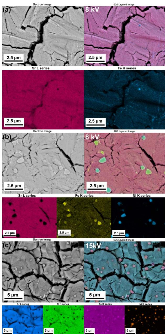
Fig. 3 Cross-sections of (a) STF reduced at 900 °C in 50% Ar/50% H<sub>2</sub>, (b) STF-N reduced at 900 °C in 50% Ar/50% H<sub>2</sub> and (c) STF-N reduced at 900 °C in 50% Ar/50% H<sub>2</sub> and reoxidized at 900 °C in air, analyzed with EDS.
