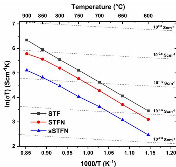
Fig. 11 Arrhenius plot of the specific conductivity for STF, STFN and sSTFN, measured at temperatures of 600–900 °C in Ar/3% H<sub>2</sub>.
