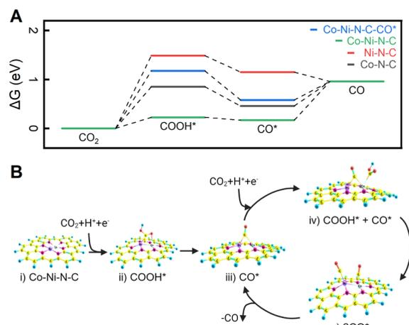
Fig. 6 (A) Calculated free energy diagrams illustrating the lowest-energy pathways to CO. (B) Catalytic pathway on the dual Co-Ni site based on the optimized structures of adsorbed intermediates COOH\* and CO\*.
