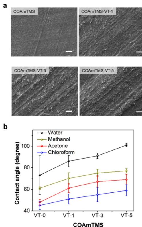
Fig. 3 (a) SEM images (scale bar corresponds to 10  $\mu\text{m}$ ) and (b) contact angle values for COAmTMS, COAmTMS-VT-1, COAmTMS-VT-3 and COAmTMS-VT-5 films in different polar and nonpolar solvents (water, methanol, acetone and chloroform).
