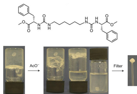
Fig. 41 Structure of a urea-based gelator used to control API crystallisation and photographs of the growth of a crystal of carbamazepine within the gel, and the use of acetate anions to disassemble the gel and allow recovery of the crystal. Figure reproduced from ref. 331 with permission of Springer Nature, © 2010.
