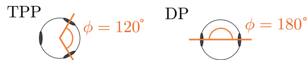
Fig. 1 TPP particles have a 120 angle and DP particles a 180 angle between their patches.
