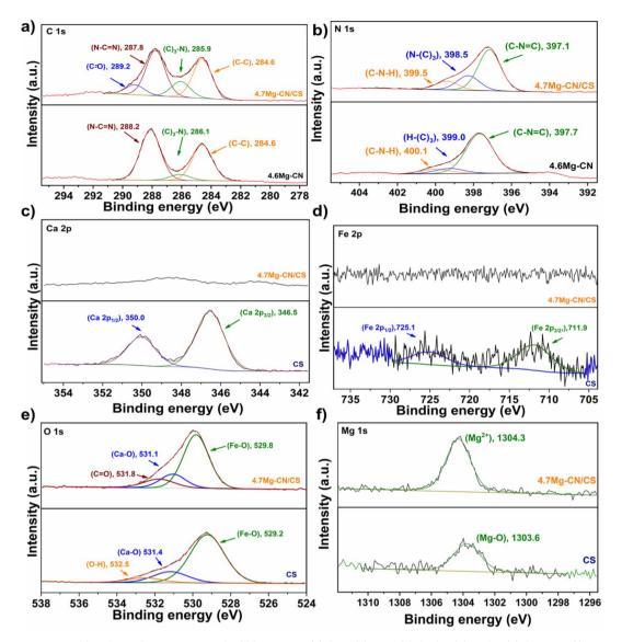
XPS spectra of the CS, 4.6Mg-CN and 4.7Mg-CN/CS samples: (a) C 1s, (b) N 1s, (c) Ca 2p, (d) Fe 2p, (e) O 1s and (f) Mg 1s.
