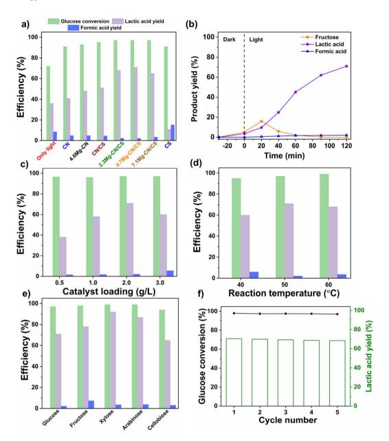
Fig. 8 (a) Glucose conversion, lactic acid yield and formic acid production by all samples; (b) product formation as a function of reaction time by 4.7Mg-CN/CS; effects of (c) catalyst dosage, (d) reaction temperature and (e) types of sugar on photocatalytic performance; and (f) reusability test of the 4.7Mg-CN/CS photocatalyst towards lactic formation in 1 M NaOH under visible-light irradiation at 50 °C after 120 min.
