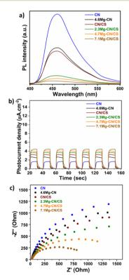
Fig. 5 (a) Room-temperature PL spectra, (b) transient photocurrent behaviour and (c) the EIS Nyquist plot of CN, 4.6Mg-CN, CN/CS and Mg-CN/CS composites with different Mg contents.
