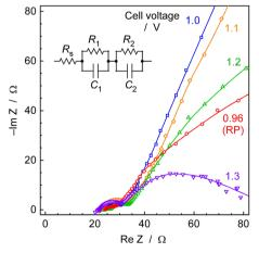
Fig. 13 Cole-Cole plots of impedance measurements at various cell voltages of hydrogen-permeable membrane cells with CsH<sub>2</sub>PO<sub>4</sub>/ SiP<sub>2</sub>O<sub>7</sub> electrolyte. The equivalent circuit of two semicircles is illustrated in this figure
