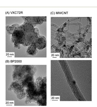
Fig. 6 TEM images of 30 wt%-Ru/Cs<sup>+</sup>(1.0)/VXC72R (A), 30 wt%-Ru/ Cs+(1.0)/BP2000 (B), and 30 wt%-Ru/Cs+(1.0)/MWCNT (C).
