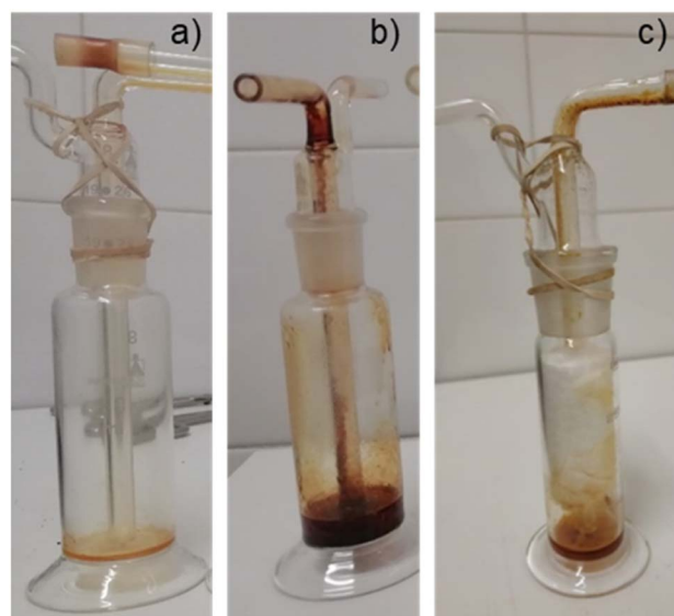
Fig. 8 Bio-oil collected in the first condenser of the experimental setup (Fig. 2) for pyrolysis of acacia (a), olive pomace (b) and eucalyptus bark (c).
