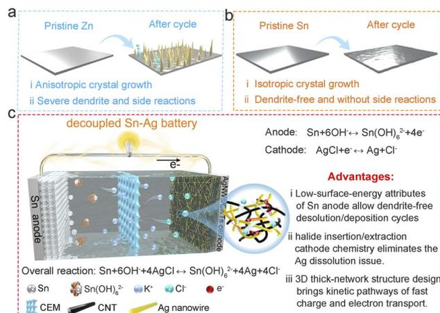
**Fig. 1** Schematic illustration of the design principles of the decoupled Sn–Ag cell. (a) Challenges of the metallic Zn electrode. (b) Advantages of the metallic Sn electrode. (c) Assembly of the decoupled Sn–Ag cell and its associated functional benefits.
