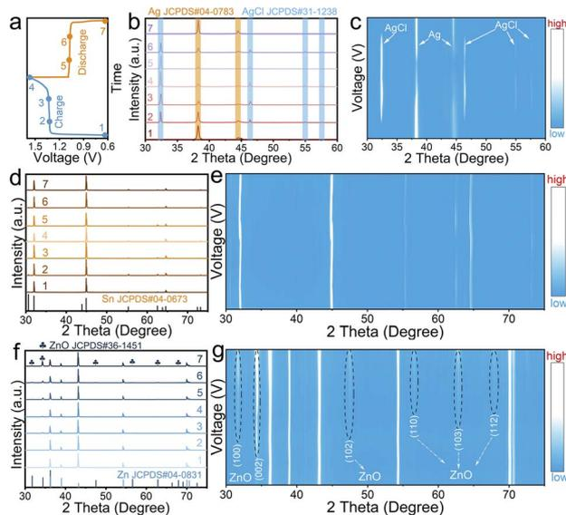
**Fig. 5** (a) The charge/discharge curves of the decoupled Sn–Ag cell recording the different charge/discharge states. The corresponding *ex situ* XRD patterns and magnified *ex situ* XRD mapping of (b and c) the AgNWs/CNT hybrid cathode and (d and e) the metallic Sn anode in the decoupled Sn–Ag cell at different charge/discharge states. (f) *Ex situ* XRD patterns and (g) magnified *ex situ* XRD mapping of the metallic Zn anode in the decoupled Zn–Ag cell at different charge/discharge states.
