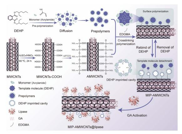
Scheme 1 Schematic illustration of the synthesis of MIP-AMWCNTs@lipase.
