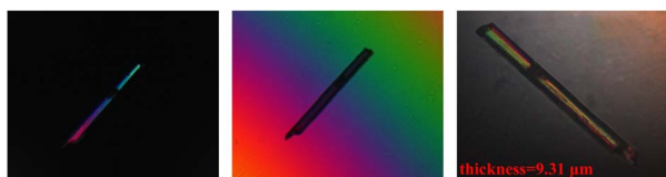
Fig. 5 Experimental birefringence at 546 nm for \text{Pb}_2(\text{SeO}_3)(\text{SiF}_6) .
